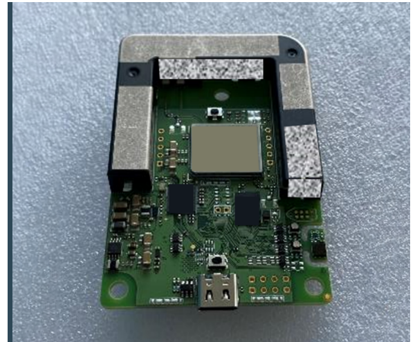
Fig. 7: Example of a U-shaped MetaSpan antenna that combines cellular, Bluetooth and GNSS antennas into a single block
