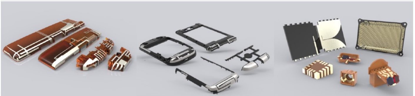
Fig. 8: Examples of LTE, GNSS and Bluetooth antennas using MetaSpan antenna and LDS technologies
